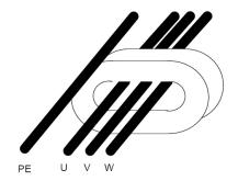
The HF-CM cores are easy to install: Simply pass the three motor phase leads (U, V, W) through the cores.
